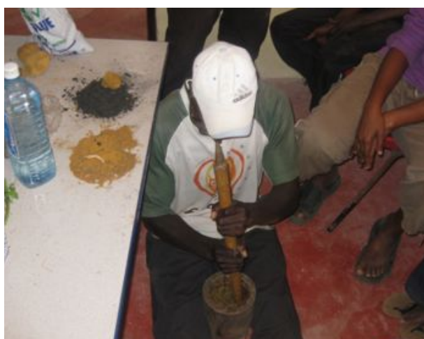
Ronald, a Vipingo caddy, grinding materials to make handmade briquettes
